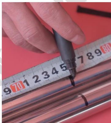
30cm 50cm 75cm 处画记号线，朝下一端画线做记号 marks the pipe with 30cm,50cm and 75cm position, marks the side for button
