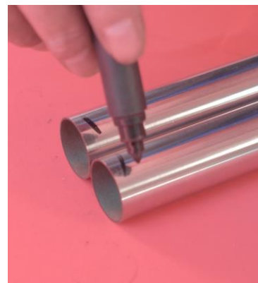
30cm 50cm 75cm 处画记号线，朝下一端画线做记号 marks the pipe with 30cm,50cm and 75cm position, marks the side for button
