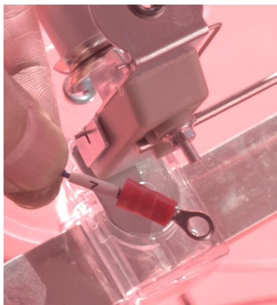
7 号报警线连接下断纱报警架 warning cable #7 connect to yarn sensor
