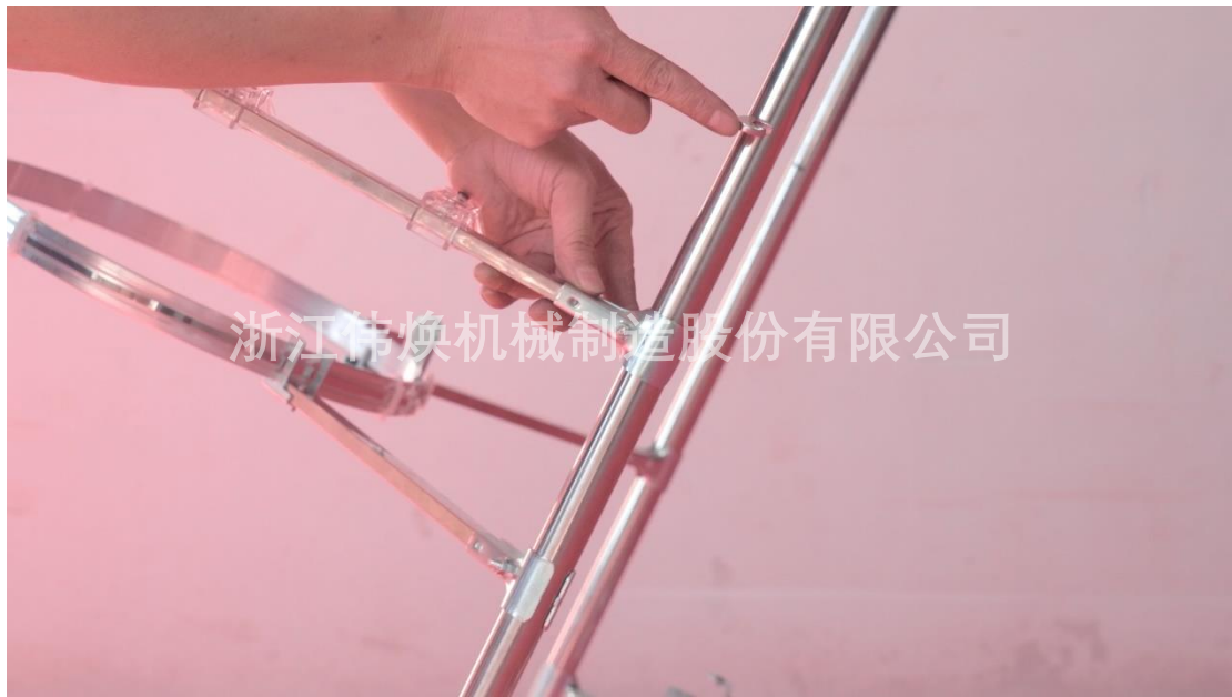
吊线过线架安装在右侧钢管 50cm 与 75cm 标记之间 the jacquard yarn holder place on the right pipe between position of 50cm and 75cm
