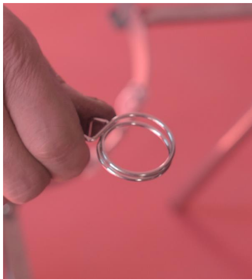
弹簧扣压紧套入钢管 75cm 标记处 put spring snap into 75cm marks position
