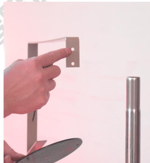
橡筋架固定在后两孔，过线板装在最上面一个孔 the elastic device fit to the table, put the elastic passing plate on top hole
